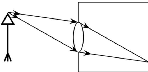
One of the advantages of using a lens over a pinhole is that a lens can bring all the light from one subject plane to a sharp focus on the film plane.
