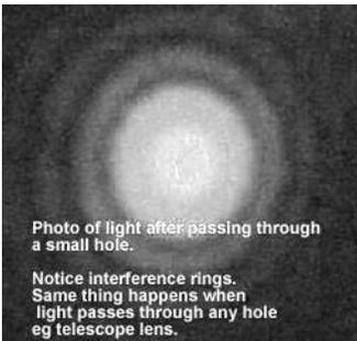
For the non-scientifically minded, this photograph of light passing through a pinhole shows the central area of light which is not scattered by diffraction, and also the concentric circles of scattered light which will cause the image to blur.
