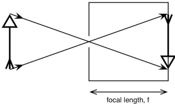
On a camera with a lens, the lens focuses light from a distant object (at infinity) at its own focal length. Moving the lens nearer to or further away from the film changes the distance at which an object needs to be in order to be brought to focus on the film.
